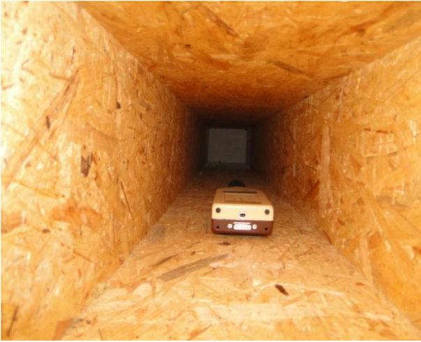
Fig. 3. Inside of the acoustic tunnel with sound level meter.
